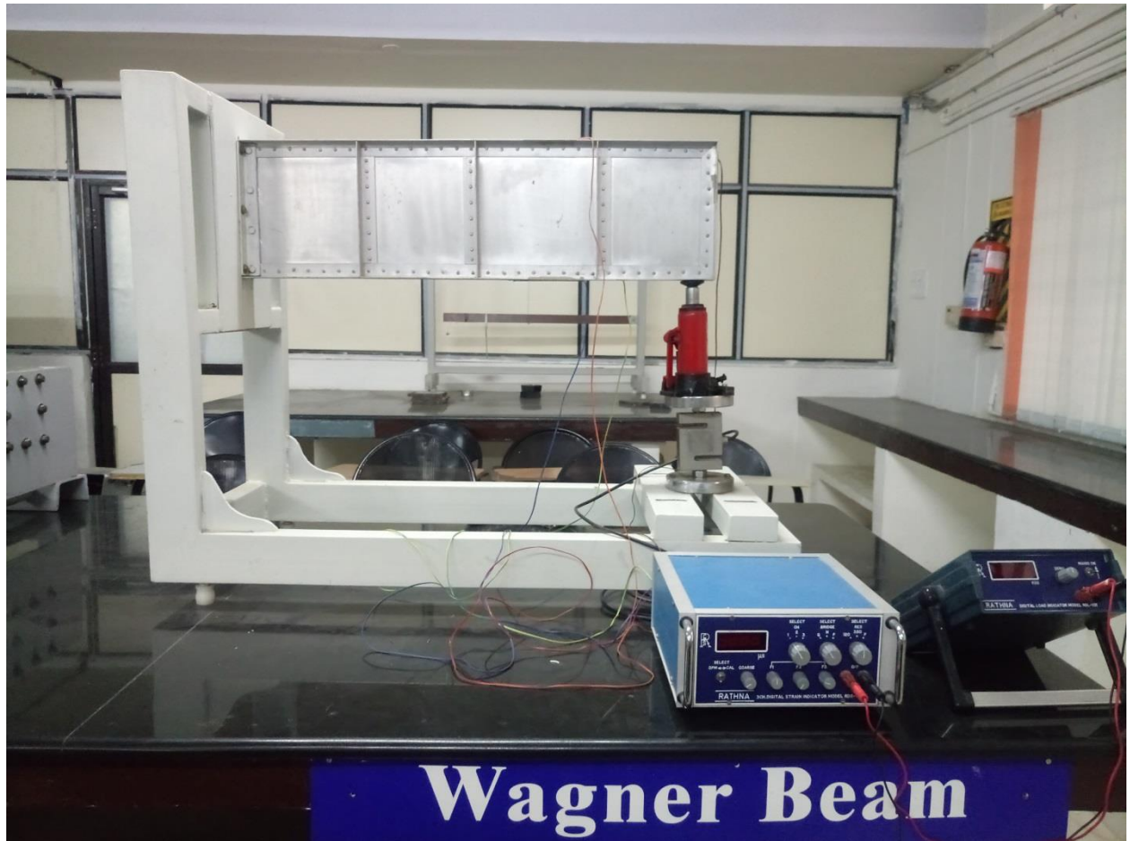
Fig.2 Wagner Beam (Aircraft wing Section hydraulically loaded with strain Gauge attached)
