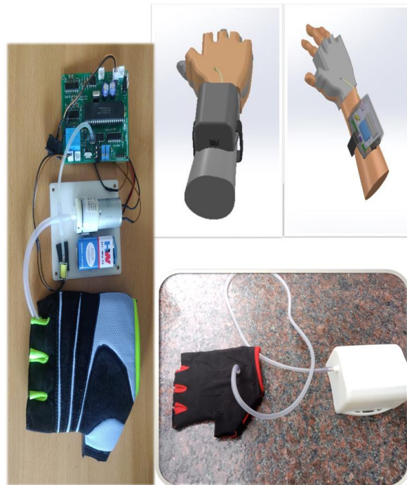
Automatic glove inflation and deflation system
