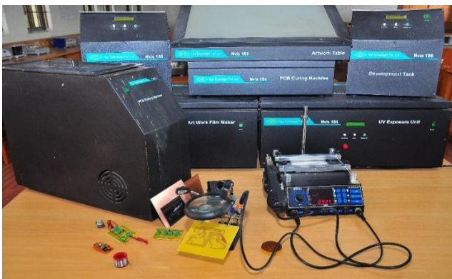
PCB Design and Fabrication System
